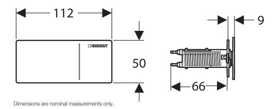
Button cannot be placed in front of the cistern. For remote Installation only. Separate service access is required to service the cistern. Button servicable from the front.
