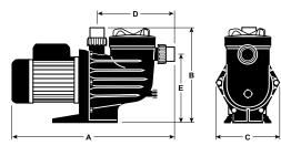
\*Suction and discharge accept 40mm PVC pipe on the I.D. and 50mm fitting on the 0.D.
