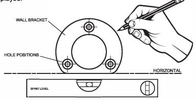
Carefully drill 7mm holes in the previously marked positions and insert the wall plugs until flush with the wall. (To ensure accuracy, we recommend to use the wall bracket as a guide and drill pilot holes using a 4mm drill bit prior to drilling the 7mm finished hole size required.)
