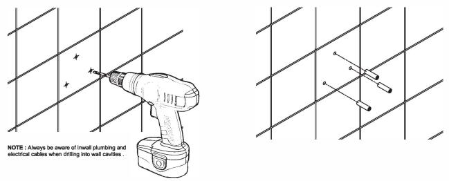
Fix the mounting bracket firmly in place using the screws supplied ensuring it is flush and firmly against the wall.
