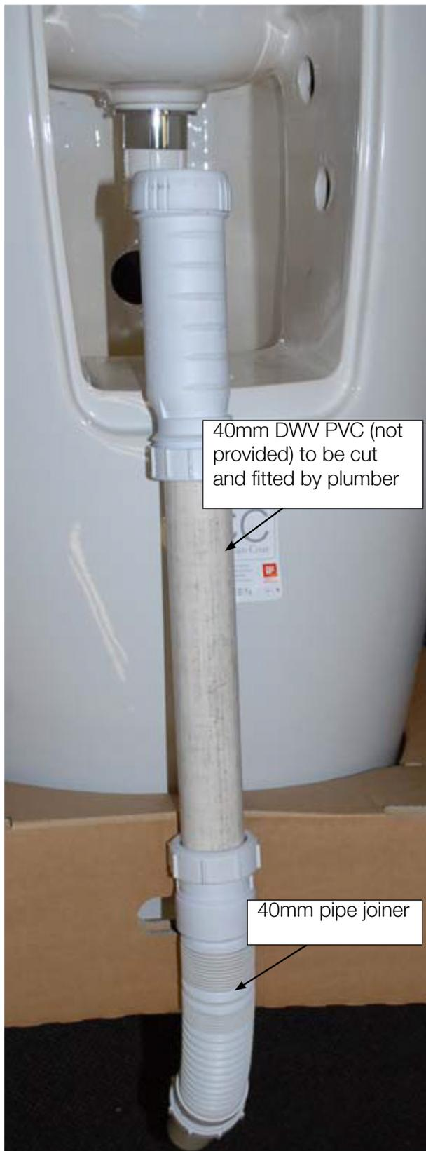
Fig. 2: Parts required between waterless trap and 40mm PVC DWV in floor.
