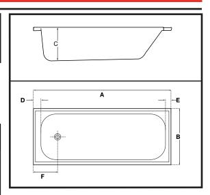
• This bath is not self supporting and does require a support at the base via Masonry, Steel or Timber (1).
