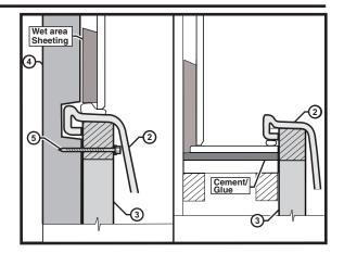
Place Bath (2) in position and connect waste. Fill Bath and then release.
