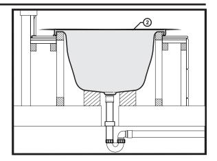
Apply Flexible Sealant (6) to the exposed edges.
