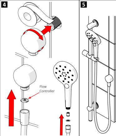
Where showers incorporate flow controllers, instructions that care be exercised during installation to ensure that the male connecting threads do not damage the flow controllers.
