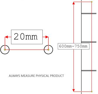
To adjust the bottom pillar, use the supplier Allen key to loosen it as shown. Move it to the required distance and tighten it securely.
