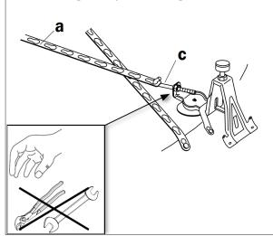
4. Turn over bath, align with the help of a spirit level by turning the screw and tighten the locknut (d).
