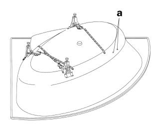
2. Slot the arm straps of the bath cradle (b) onto the lugs (a) on the base of the bath.
