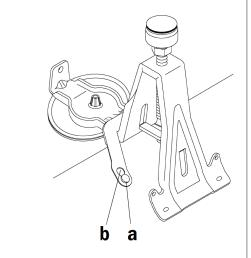
Push a suitable length of the tensioning belt onto the retaining bolt (a), engage the threaded hook (c) and tighten by hand using the nut on the base.
