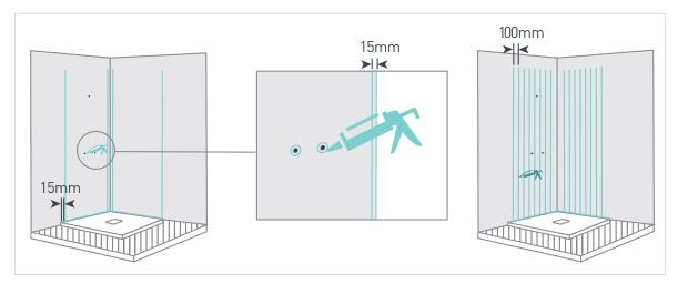
• Before fitting the shower wall, apply a bead of silicone sealant supplied along the inside face of the tile bead upstand of the shower base as shown below.
