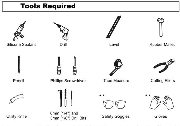
\* Use the correct type of drill bit for the material being drilled, with 6mm required for anchor fixing and 3mm used for screwing directly into the wall studs.
