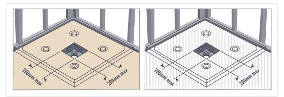
• Before the shower base can be installed, the choice of wall construction and wall lining method must be determined. The choice will determine which of the following methods should be followed:
