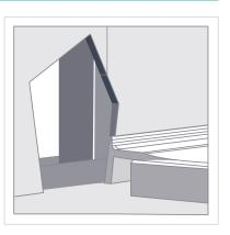
• Once sheeting is completed, use a flexible waterproof sealant (not supplied) to seal the gap between the shower base tile bead and the wet area sheet.
