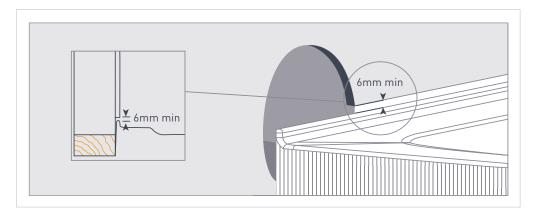
Once sheeting is completed, use a flexible waterproof sealant (not supplied) to seal the gap between the shower base tile bead and the wet area sheet.
