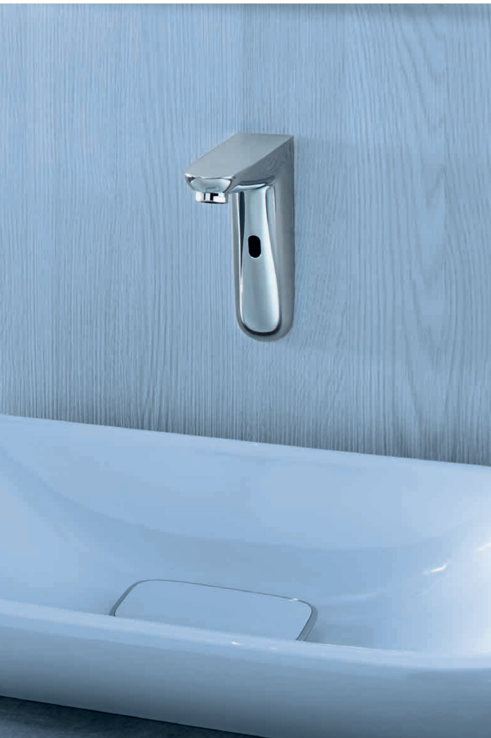
121 570 Infrared Basin Mixer (6 V) wall-mounted without mixing device projection: 170 mm WELS 6 stars, 4.5 ltrs/min
