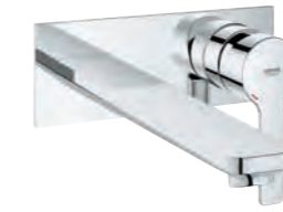
23 839 001 + 23 842 000 Wall mounted Basin Mixer set L size + separate concealed body Projection: 207mm WELS 5 stars, 6 ltrs/min
