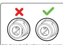
Note: Always check the rubber seal on the ceramic Cartridge is a round uniform shape. If distorted push back into place or the cartridge will leak when water is introduced.
