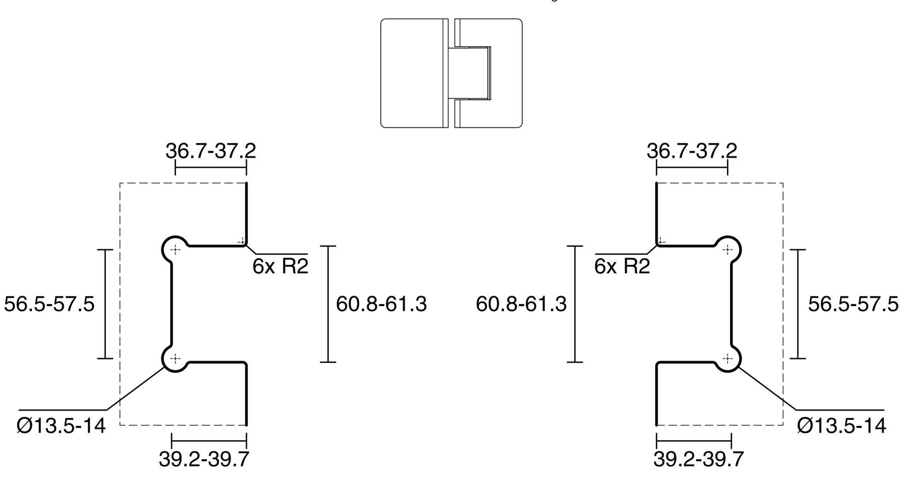
Please note that the cutout template is provided as a guide only. This cutout template should be checked against the actual screen to determine correct fit.
