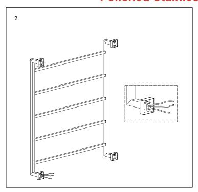
• Connect the power chord to the power supply.
