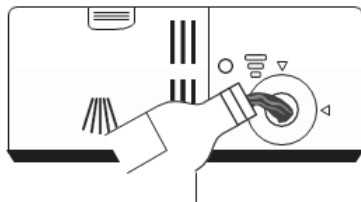
Figure 10- Filling the Rinse-aid reservoir.
