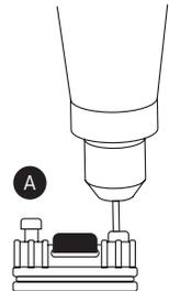
6. Flip the top part of the clip over on top of the pool cover. Using the screwdriver, let the 2 screws pierce through the cover, securing the cover onto the clips. Repeat for all clips.
