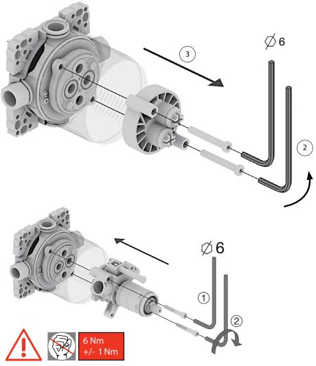
Tighten the 2 screws parallel (1 turn each side) Check before installation that all seals are available and at the right place
