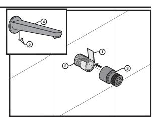
Insert the Bath Outlet (4) body to the Outlet Adapter (3) and resecure the Grub Screws (5).
