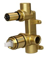
The Mizu Universal Inwall Body is an innovative installation system that separates the inwall body from the trim kit. Install the Universal Inwall Body during rough-in and leave the tapware colour choice for later.
