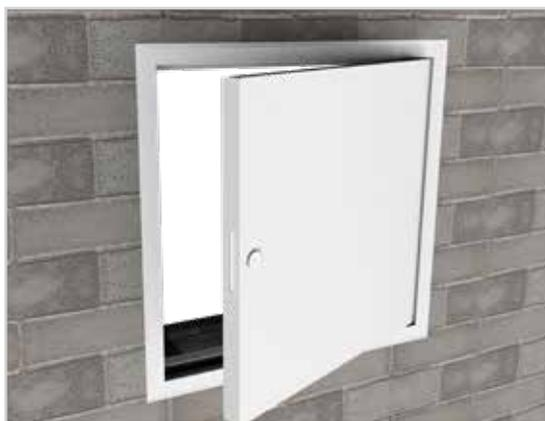
With the door open, screw the frame into the wall/ceiling through the pre-formed fixing holes provided (400mm centres recommended).
