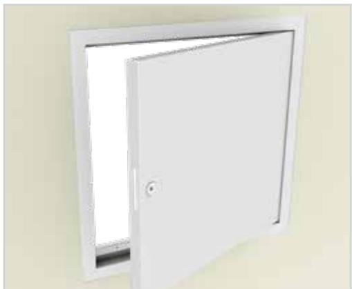
With the door open, screw the frame into the wall/ceiling through the pre-formed fixing holes provided (200mm centres recommended).
