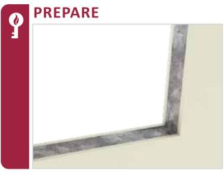
The opening must be framed with studs/ noggings to affix the panel to.
