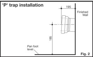
IMPORTANT: ALL DIMENSIONS ARE TO THE UNDERSIDE FOOT LEVEL
