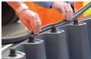
5. Inset profile seal and centring bolts
