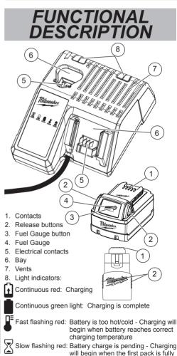
charged Flashing red/green: Damaged or faulty battery pack
