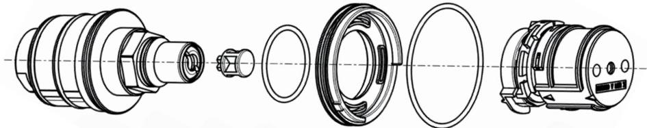
6. Unscrew cartridge with a 24mm A/F deep socket, expect some trapped water to escape. Replace the cartridge if necessary. When refitting cartridge, do not over tighten, hand tighten the first few threads, maximum torque 16Nm.
