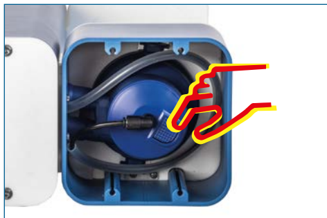
Fig. 6: Setting head for water blending.
