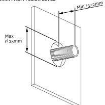
Install a ½" male threaded connection at the recommended height on wall, ensuring that a minimum of 13±2mm of thread protrudes past the finished wall.
