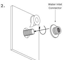
Loosen the 2 grub screws with the Allen Key supplied and remove Water Inlet Connector from diverter. Apply thread tape (or Similar) to the ½" connection and screw Water Inlet Connector onto the ½" connector.
