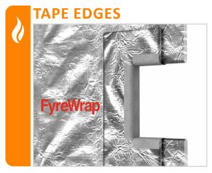
Tape the edges of both layers of FyreWrap® Elite 1.5 together.
