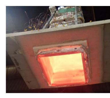
Note: FyreWrap® Access Panels are tested for internal fire applications only.
