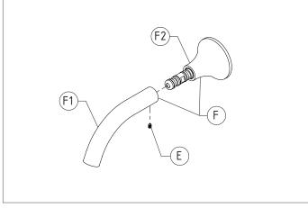
14) Ensure the area is clean and clear of debris. Seal the wall penetration and apply teflon tape or alternative sealant to the wall breech thread.
