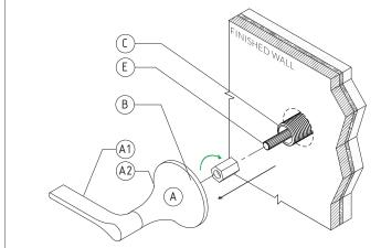
12) Re-fit Spindle Hex Adapter (B) and Handle Assembly (A) Repeat step 9-12 until horizontal handle alignment is achieved.
