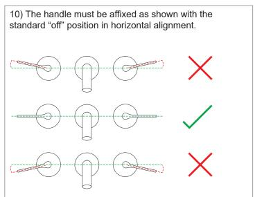
11) If the handle alignment is not correct, remove the Handle Assembly (A) and Spindle Hex Adapter (B) and rotate to engage a different position on the spline.
