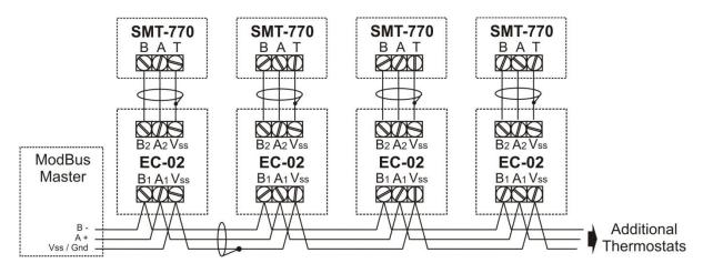
The Last EC-02 may require the End Of line (EOL) resistor in circuit.
