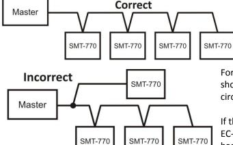
When wiring the SMT-770, it is important that you use screened cables. All screens should be joined together and grounded in 1 location only.
