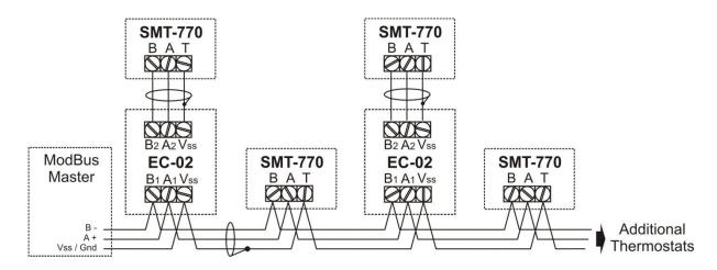
The last device in the network may require the End Of Line (EOL) resistor in circuit.
