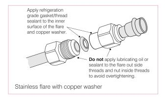
Align the centers of both flares and tighten the flares by hand.
