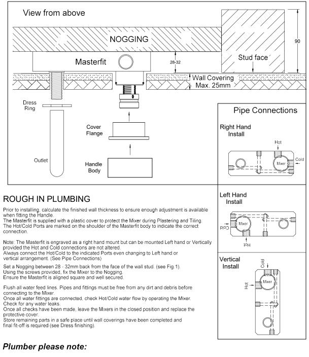
On-site high pressure line testing must be conducted with the Mixer in the closed position. (STATIC TEST ONLY) Under no circumstances is the Mixer to be opened when exceeding the maximum stated water pressure. At the completion of the testing, do not relieve any high pressure by opening the Mixer. Exposing the internals of the Mixer Cartridge to higher than specified water pressures, will void the manufacturer's warranty.
