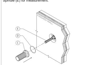
4) Measure the amount of Locknut (C) thread protruding from the finished wall and mark between 15-20mm.
