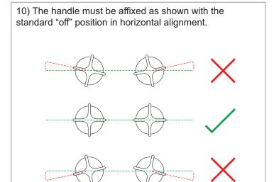
11) If the handle alignment is not correct, remove the Handle Assembly (A) and Spindle Hex Adapter (B) and rotate to engage a different position on the spline.
