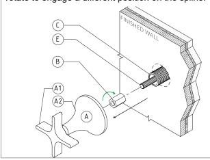
12) Re-fit Spindle Hex Adapter (B) and Handle Assembly (A) Repeat step 9-12 until horizontal handle alignment is achieved.
