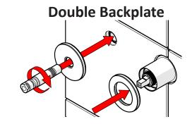
Gently push Dress Plate over Wall Mixer Sleeve. Align outlet hole in wall with outlet hole in Dress Plate. Fasten Spout Adaptor through Dress Plate onto in-wall Mixer Body.
