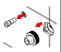
Add grease or soap to Cartridge Legs. Push Cartridge gently Into Body. Ensure correct
