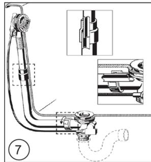
1/2" Dual Check Valve supplied must be installed to inlet connection to meet AS/NZS 3500 requirements - use thread seal tape or equivalent
