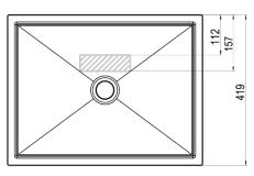
NOTE: (Grey area) The optimum area of water impact for a tap with a vertical outlet
