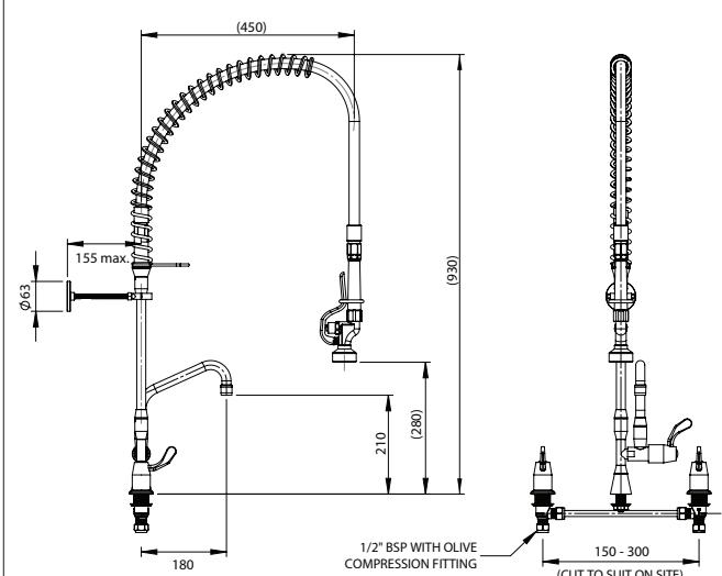
Spray trigger position dimensions are approximate and represent a brand new unit, spring will sag with use over time
