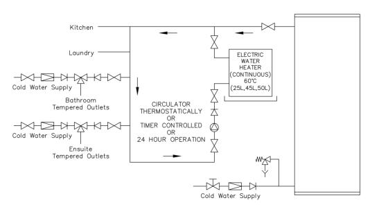
NOTE: A PLV IS REQUIRED TO BE INSTALLED ON THE COLD SUPPLY LINE TO THE TEMPERING VALVE IF A PLV IS INSTALLED ON THE COLD SUPPLY LINE TO THE WATER HEATER.
