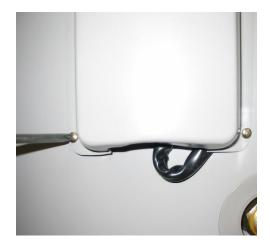
Step 2 remove screws from lower front cover
