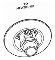
Step 13 attach flexible hose with blue stripe to inlet and ball valve in open position
