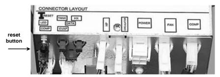
2. The green LED will flash rapidly for three (3) seconds, then the heat pump will commence its heating start-up cycle. A series of 2 or 3 x green flashes will commence.
