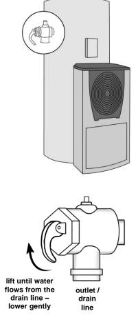
Operate the easing lever on the temperature pressure relief valve and expansion control valve once every six (6) months to clear any deposits and ensure the valve and its drain line are not blocked. It is very important the lever is raised and lowered gently. Refer to "Minor Maintenance Every Six Months" on page 15.
