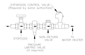
A disconnection union must always be provided at the cold water inlet and hot water outlet on the water heater to allow for disconnection of the water heater.
