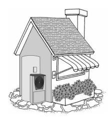
The water heater is to be installed at ground or floor level and must stand vertically upright on a stable base, as acceptable to local authorities, of a minimum size 900 mm wide x 650 mm deep. The heat pump module must be fully supported by the stable base.
