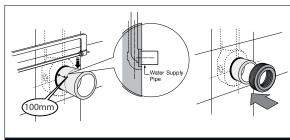
Water inlet pipe should be roughed in at 380mm. Cut inlet pipe so that 100mm protrudes from finished wall and attach seal.
