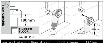
Insert waste pipe into floor at a setout of 95-110mm and 180mm above finished floor and fix bracket into position as per diagram above.
