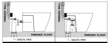
Push pan into position. Ensure that you make a firm connection with inlet and outlet pipes and avoid disturbing the floor fixing brackets. Flush test for leaks
