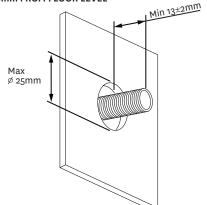
Install a  $\frac{1}{2}$ " male threaded connection at the recommended height on wall, ensuring that a minimum of  $13\pm2$ mm of thread protrudes past the finished wall.
