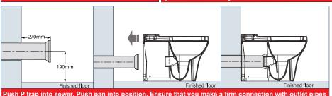
Push P trap into sewer. Push pan into position. Ensure that you make a firm connection with outlet pipes and avoid disrupting the floor fixing brackets. Flush test for leak
