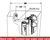
using 15 mm M + F ball valve supplied
