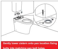
bolts into matching pan bolt holes
