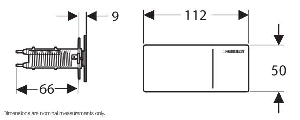
Button cannot be placed in front of the cistern. For remote Installation only. Separate service access is required to service the cistern.
