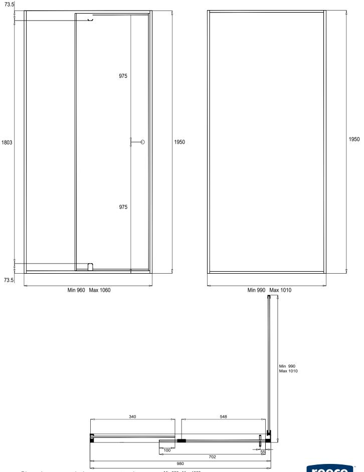
Dimensions are nominal measurements only. Dimensions are shown in Millimetres
