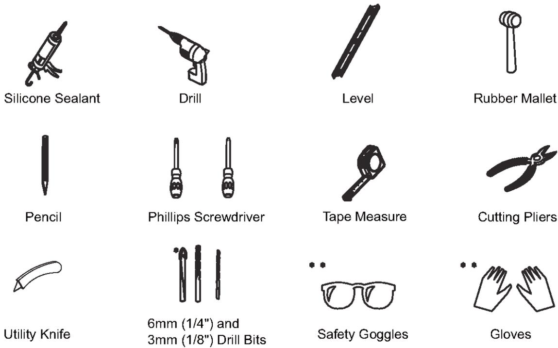
\* Use the correct type of drill bit for the material being drilled, with 6mm required for anchor fixing and 3mm used for screwing directly into the wall studs.
