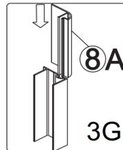
Slide both section together then attach to return Panel
