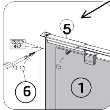
Before fixing of this rivet or screw, make sure door glass is level and in line with head rail
