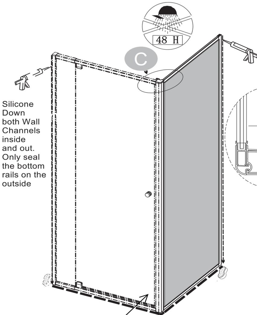
Silicone Down both Wall Channels inside and out. Only seal the bottom rails on the outside
