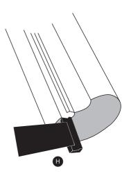
**9.** Insert the tube into the tube ends.
