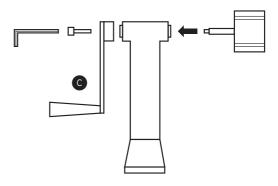
4. Screw the roller lock (D) onto the roller end, be sure to use the side with the roller handle. The black screw that was removed in the first step can be screwed back into the end without the roller lock.
