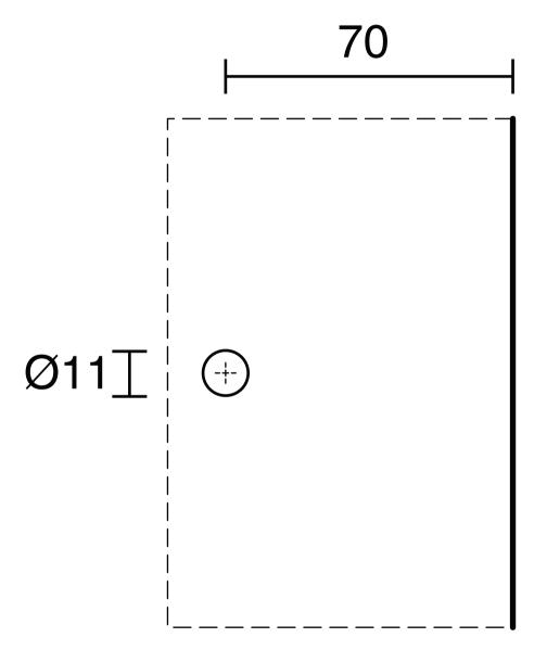
Please note that the cutout template is provided as a guide only. This cutout template should be checked against the actual screen to determine correct fit.
