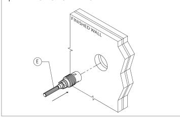
2) Once Fitted, Ensure both spindles (E) are set to OFF position - HOT = FULL TURN CLOCKWISE and COLD = FULL TURN ANTICLOCKWISE.
