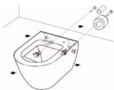
(Fig.5) Insert pan fixing plugs and push back onto fixing bolts.
