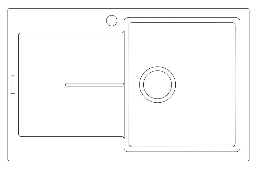
Please note that the cutout template is provided as a guide only. This cutout template should be checked against the actual sink to determine correct fit.
