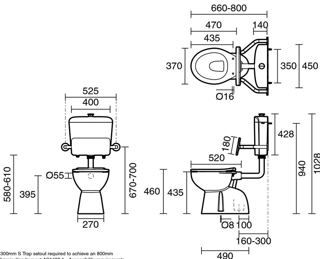
Note: 300mm S Trap setout required to achieve an 800mm overall projection to meet AS1428.1 - Accessibility requirements
