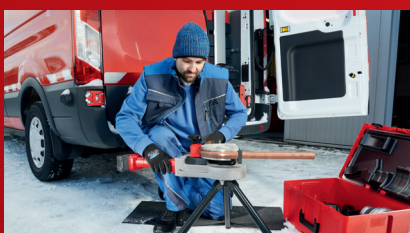
Pre-adjustment of the bending angle without tools
