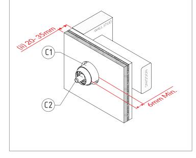
3) Slide the Dress Ring (B) over the Wall Mixer Sleeve (C1) to meet the finished wall. Fit Handle (A) onto the cartridge lever (C2).
